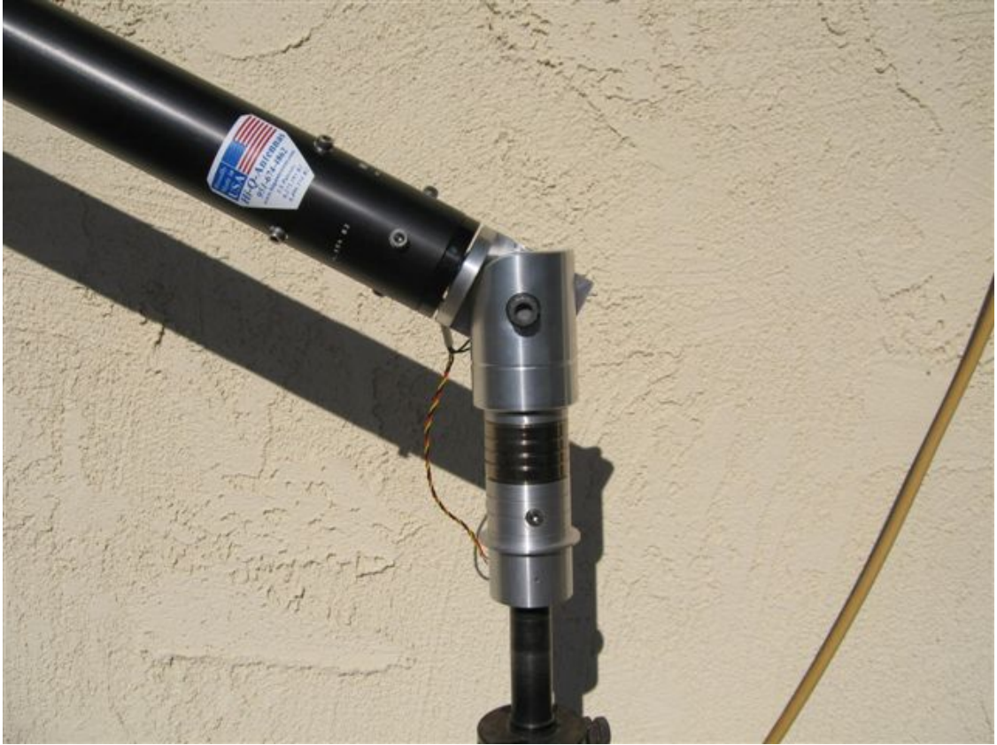
Hi-Q™ Fold-over base at 30 degrees
